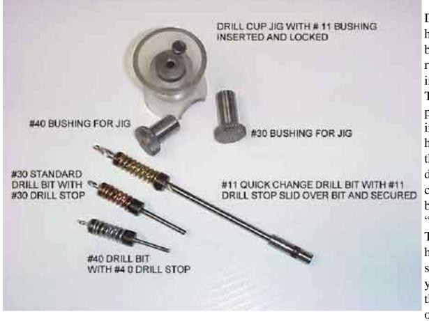
Drills, drill bits and holes. An aircraft is basically thousands of rivets and bolts flying in close formation. These squeeze various parts together, inserted through holes, many of which the builder has to drill. The industry calls these rivets. bolts. screws etc. "fasteners". The drilling of these holes is quite an exact science, and how well you drill them affects the structural integrity of your aircraft (now
