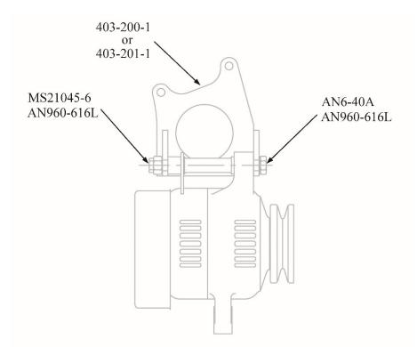
Step 4. Connect the 403-200-1 or 403-201-1 bracket to the lug on the inboard side of the starter using an MS20074-05-05 bolt and AN960-516L washer. Torque to 150 +/- 15 in-lbs.
