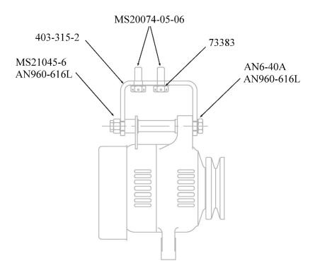
Step 3. Mount the 403-315-2 bracket to the engine case boss, using the two MS-20074-05-06 bolts and the 73383 locking plate. Torque the bolts to engine manufacturer's specifications or 110-150 in-lbs. Lock the bolts by bending the tabs on the locking plate up against the flats on the bolt hex.
