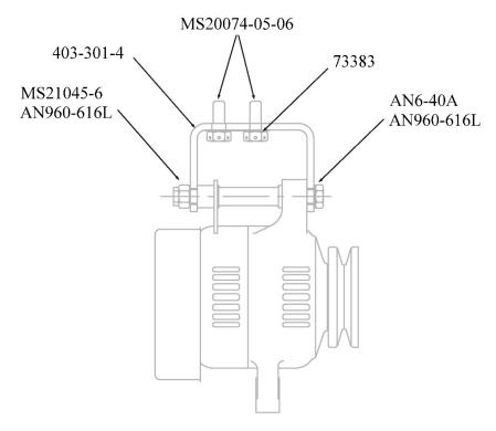
Step 4. Position the LX60 alternator so that the alternator "pivot tube" fits within the U-shaped opening of the 403-301-4 bracket. Secure the alternator in place using the AN6-40A pivot bolt, two AN960-616L washers, and MS21045-6 locking nut. Do not fully tighten bolt and nut to allow for later adjustment.
