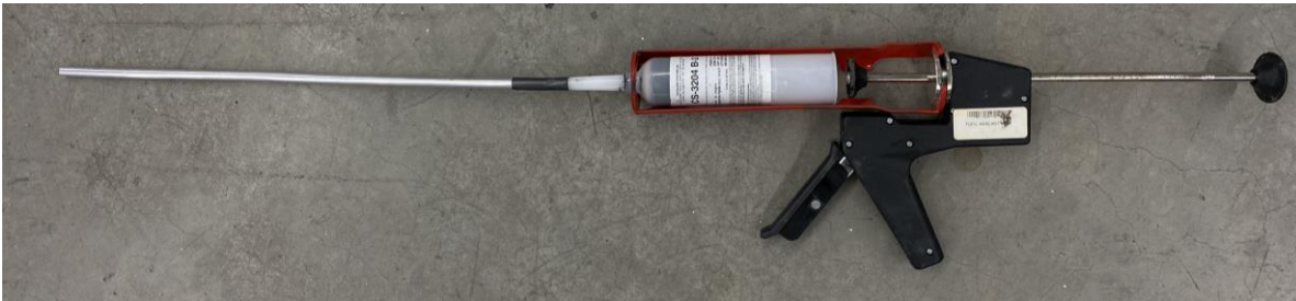
FIGURE 8: SEALANT GUN WITH 3/8 ALUMINUM TUBE ATTACHED WITH TAPE TO NOZZLE OF MC-236-B1/2 FUEL TANK SEALANT CONTAINER
