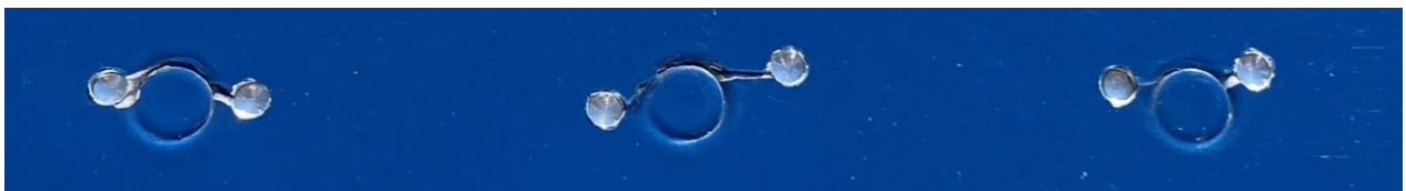
FIGURE 3: STOP-DRILLED CRACKS ON RV-14A ELEVATOR
